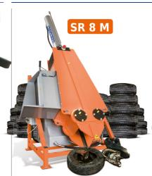
This machine is designed to separate the tire from the rim in an easy and safe way. The wheelspress reduces the volume of the iron and press it ready for furnaces. The wheelspress can crush from 80 to 140 wheels per hour, that means approximately 32 / 55 qt of iron per day. For this reason this machine gives a quick Return of Investment (ROI).
