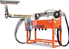
Brakes oil drainage, engine oil drainage, gear box oil drainage, windscreen-wiper water drainage, radiator's water drainage.
